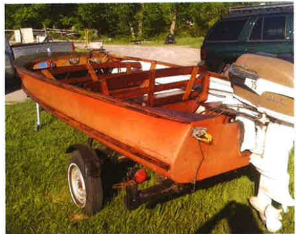
Don Husak's early Peterborough fiberglass was made in a mould taken from a 1950's Peterborough cedar strip.
