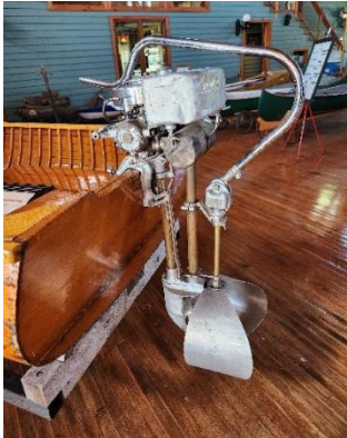
1929 Johnson with McNab reversing rudder device.
