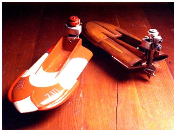
These two outboard hydroplane tether boats are powered by fuel burning, glow plug, toy outboards. The boat on the right has an Allyn Sea Fury two-cylinder motor, the boat on the left has an Atwood single cylinder. These glow plug toy outboards are from the mid 1950's. Fuel burning motors were very fast, no comparison to the slower battery operated and clockwork toy outboards.
