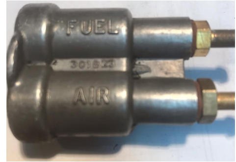
2-line connector.. see "Air" cast in.
