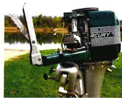
Dave Kennedy's 4 cyl MERC Thunderbolt with dead man's throttle control.
