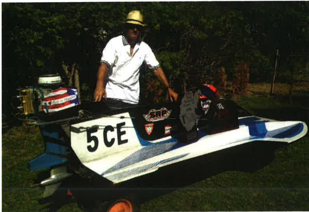
Rob Dixon, APBA National Champion, with his Sidewinder hydro & Merc "A" stock motor. This outfit has a top speed of 58 mph.
