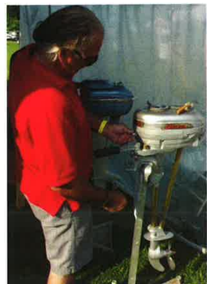
Admiration for the 1940's Lauson, air cooled, 4 cycle, single
