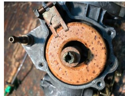
**New float, new needle & seat, new main metering nozzle gasket installed.**
