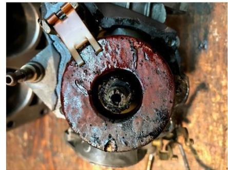
**Destroyed float and main metering nozzle covered in tar deposits**
