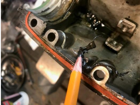
Excessive "Right Stuff" slopped all over the inside of the skeg
