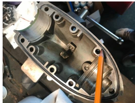
Skeg all cleaned, groove all cleaned, new Cord laid in groove & affixed with 3M, 847 adhesive
