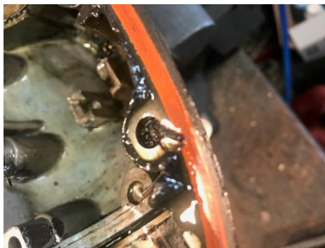
Orange silicon seal spread in the skeg groove., The proper BUNA rubber cord seal was missing.
