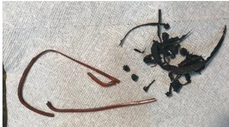
The garbage remnants of the black "Right Stuff" & the semi-cured Orange silicon seal that were removed from and around the skeg.
