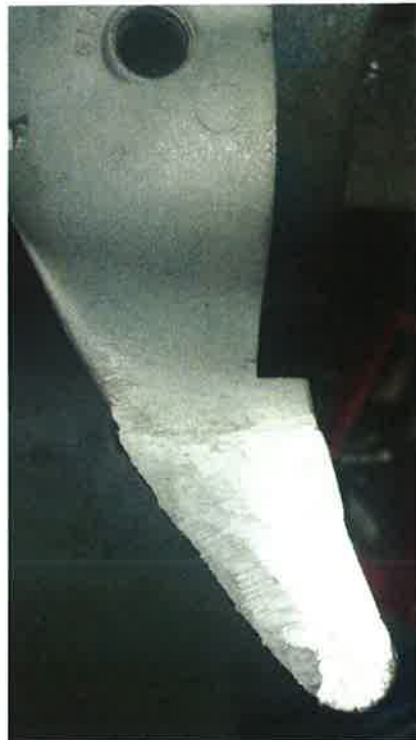
Right: Excess metal ground away close to final size.
