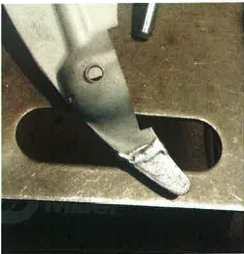
Above: Replacement skag welded in place.
