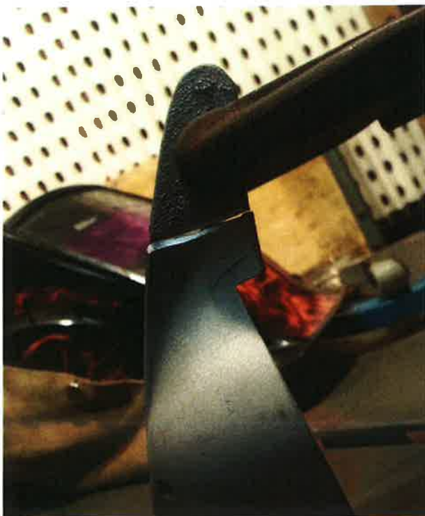
New piece, cut to size and held in place ready to tack weld.
