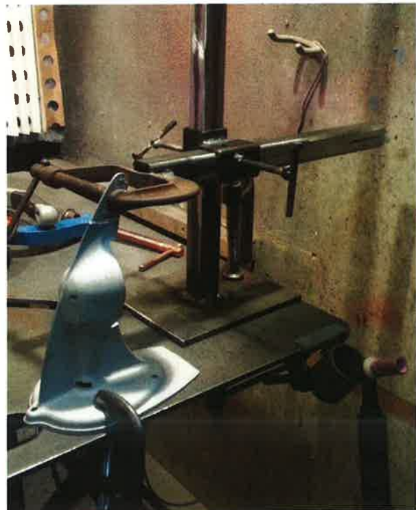
View of "Third Hand" I made to hold parts for welding.
