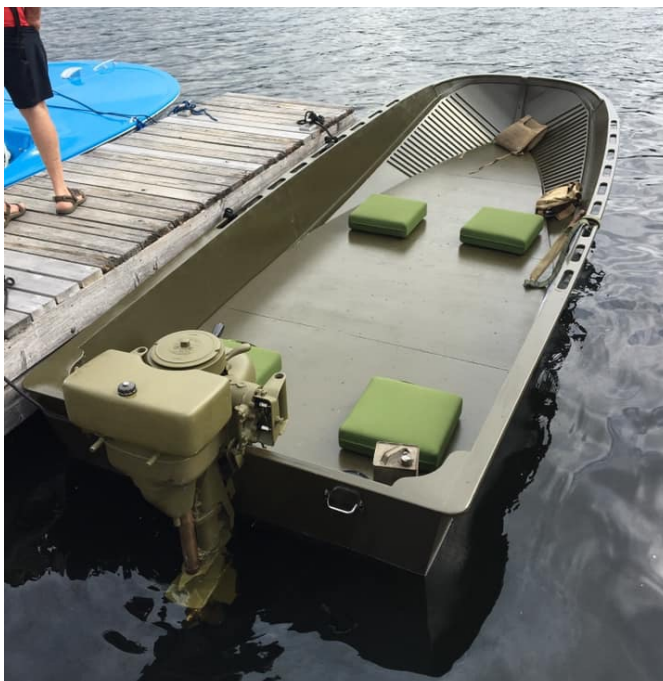
Ron Stevenson's recreated Storm Boat with restored Evinrude Storm Boat Motor.
