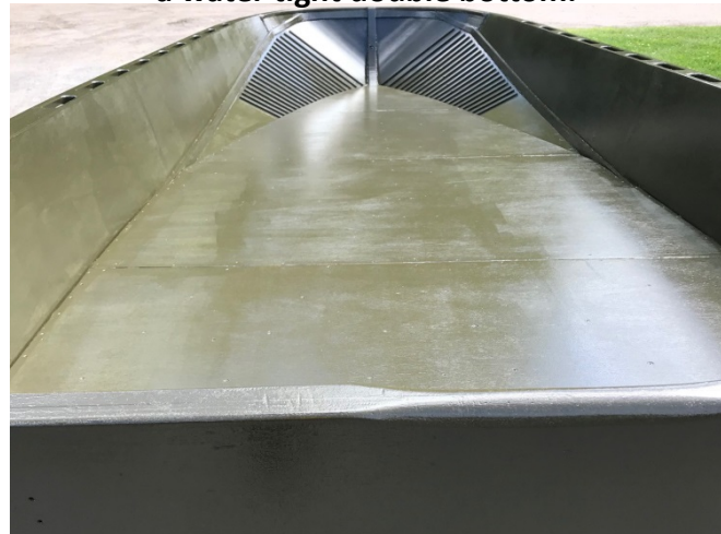
Bottom framing was designed to form water tight compartments & superior strength. Flat floor over the framing created a water tight double bottom.
