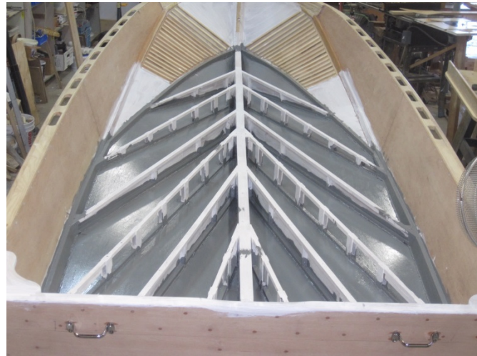
Bottom framing was designed to form water tight compartments & superior strength. Flat floor over the framing created a water tight double bottom.
