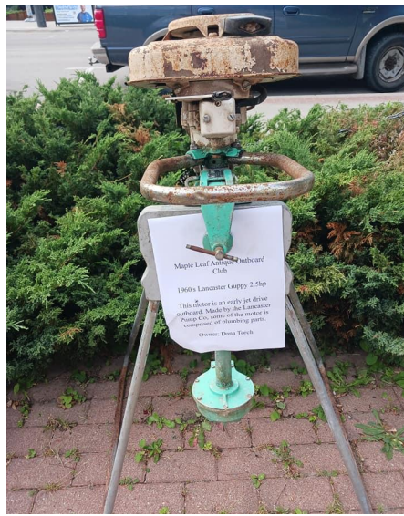
Dana's 1960's Lancaster "Guppy", an early jet drive outboard.
