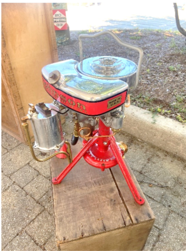
Sandy Kennedy's Johnson powered Belle Mead Fire Pump.
