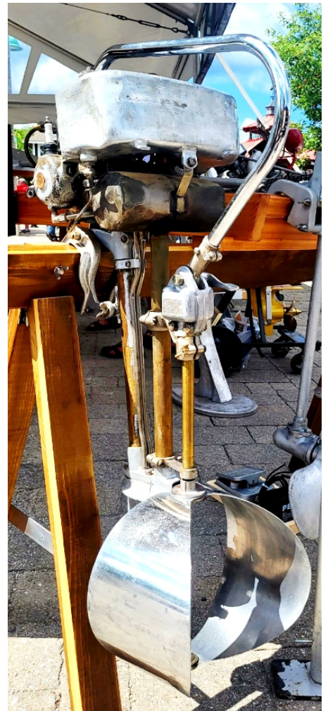
Terry Philpots' early Johnson with rare McNabb reversing rudder devise.
