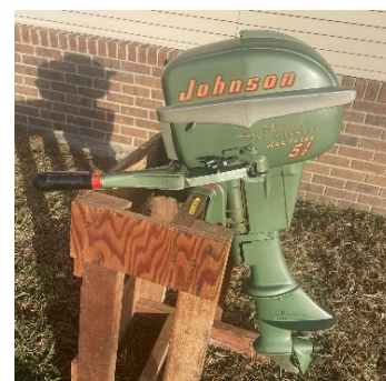
(Fig.8) The port side of a CD-10. Note the lack of arm on the throttle gear & the cowl is not cut away for clearance.
