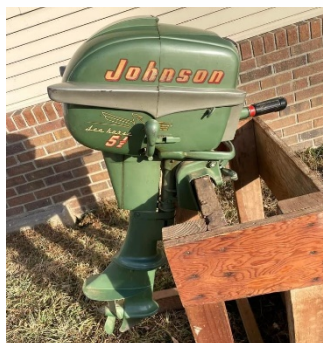
(Fig. 7) The starboard side of a CD-10 showing the early design shift handle, not compatible with remote control.
