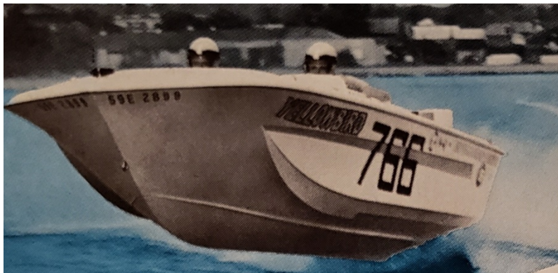
"Yellowbird" 766 was a Chrysler Hydro-V hull powered by twin Chrysler 105 outboards. Driven by Jerry Rice, this combo was Canadian High Points Champion, U2 Sportcraft Division, 1968, 69 & 70.
