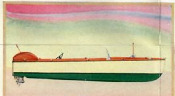
Electric Starting Aquaflyer 17 1/2-ft. De Luxe Runabout Sealite construction, V bottom, 5 ft. beam; sporty double cockpit arrangement, with two upholstered cross seats with lazybacks; weighs 450 lbs.; true speed up to 19 m.p.h. with Sea Horse "16"—up to 25 m.p.h. with Sea Horse "32."
